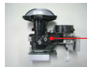
Key optical parts are shielded for dust protection.
