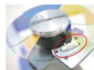
Magnetic sensor is effective against dust.
